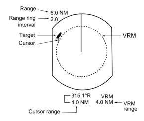
Figure 2-5 Measuring Range by the Cursor and the VRM
